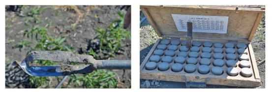
Figure 2. Equipment for gravimetric soil moisture measuring *Source:* photo by the authors
