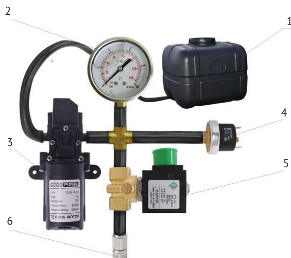
Figure 2. Connection diagram of devices for determining the required nozzle diameter and operating pressure for creating a stand, where 1 – tank; 2 – pressure gauge; 3 – water pump; 4 – pressure sensor; 5 – actuator; 6 – nozzle
