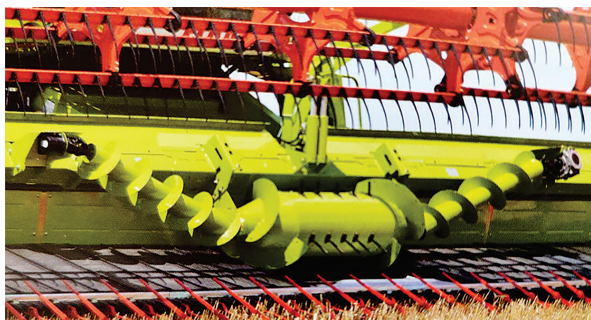
Figure 5. Equipment for uniform mass distribution
