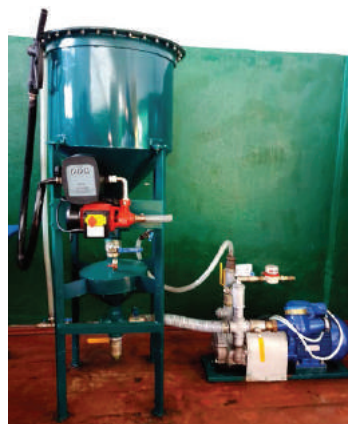
Fig. 1. The circulation mixer-separator for vegetable oil transesterification
