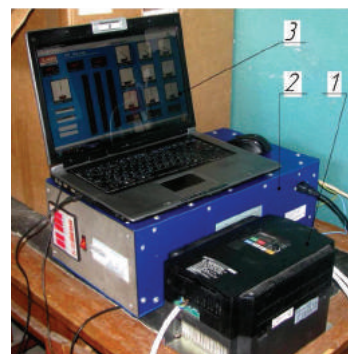
Fig. 2. Measuring equipment: 1 – frequency inverter; 2 – digital power consumption meter; 3 – laptop with special software installed
