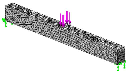
Fig. 3. Grid of finite elements of a straight-line beam patterned from pre-deformed lamellae
