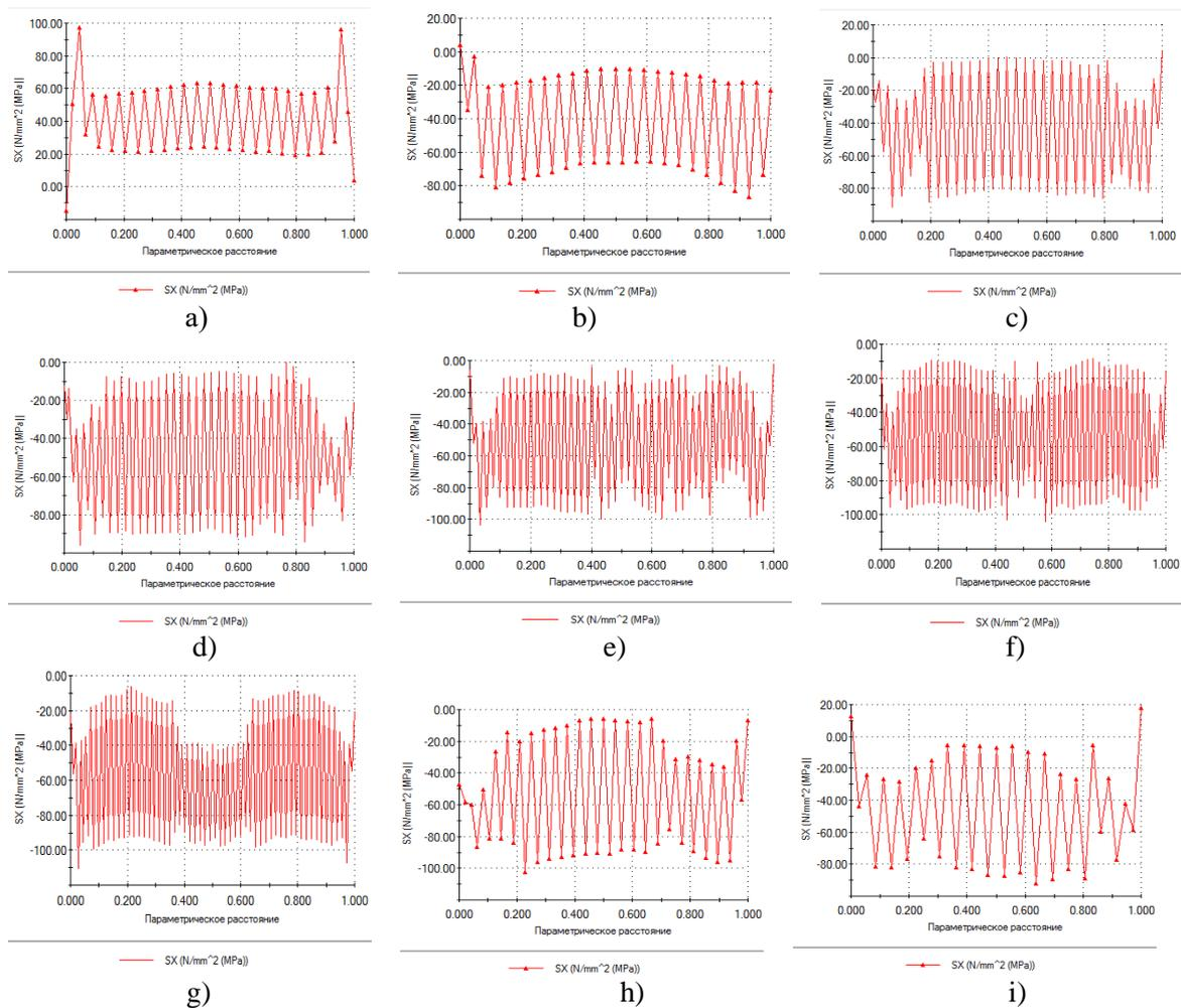
**Fig. 9. Parameterized graphs of normal stress at design points of finite elements: a – the lower edge of the first lamella; b – second lamella; c – the third lamella; d – fourth; e – fifth; f – is the sixth; g – the seventh; h – the eighth; i – the ninth.**
