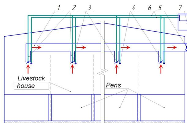
**Figure 1.** Technological scheme of automatic ventilation system for polluted air intake: 1 – central air duct; 2 – branch pipes; 3 – intake dampers with servomechanisms; 4 – temperature, humidity, and air quality sensors; 5 – exhaust fan; 6 – electrical wires; 7 – control unit
