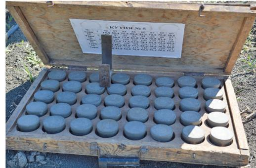
**Figure 2.** Equipment for gravimetric soil moisture measuring
