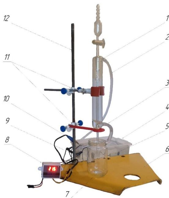
**Figure 1.** Installation for determining the kinematic viscosity of the oil at a given temperature: 1 – viscometer, 2 – feed tube, 3 – drain tube, 4 – water tank, 5 – pump, 6 – stand, 7 – working fluid sample tank, 8 – thermostat, 9 – temperature sensor, 10 – electric heater, 11 – viscometer holders, 12 – rod
