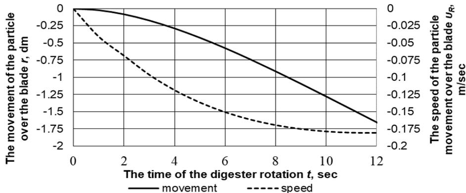
Fig. 5 - The dependence of the movement over the digester blade and the speed of the organic particle on the rotation time (angular velocity of the digester rotation  $\omega=0.1$  rad/s, inner radius  $R=2$  dm)
