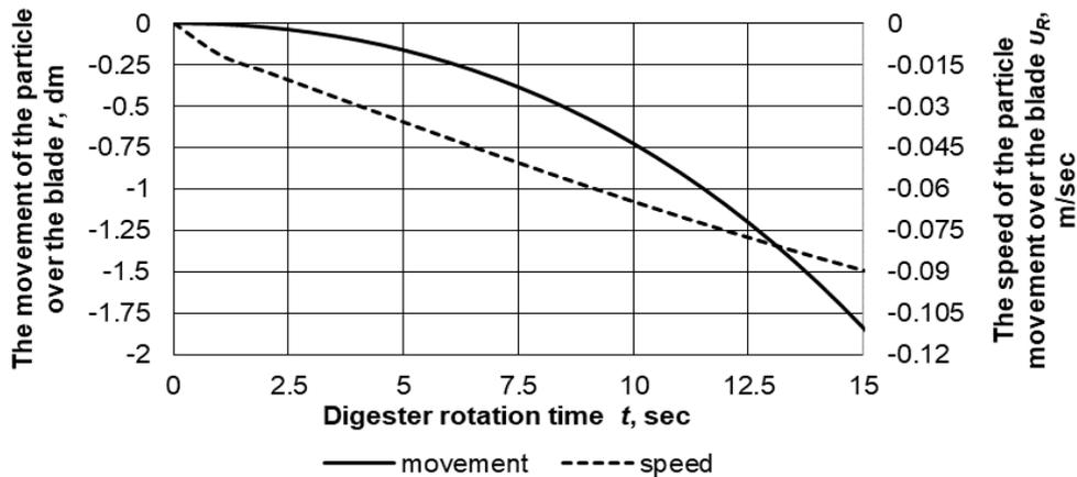
Fig. 4 - The dependence of the movement over the digester blade and the speed of the mineral particle on the rotation time (angular velocity of the digester rotation  $\omega=0.1$  rad/s, inner radius  $R=2$  dm)
