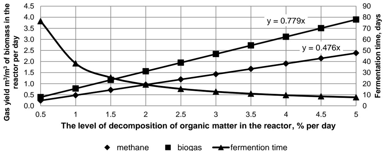
Fig. 4 – The effect of organic matter decomposing intensity on the specific yield of biomethane, biogas and fermentation time
